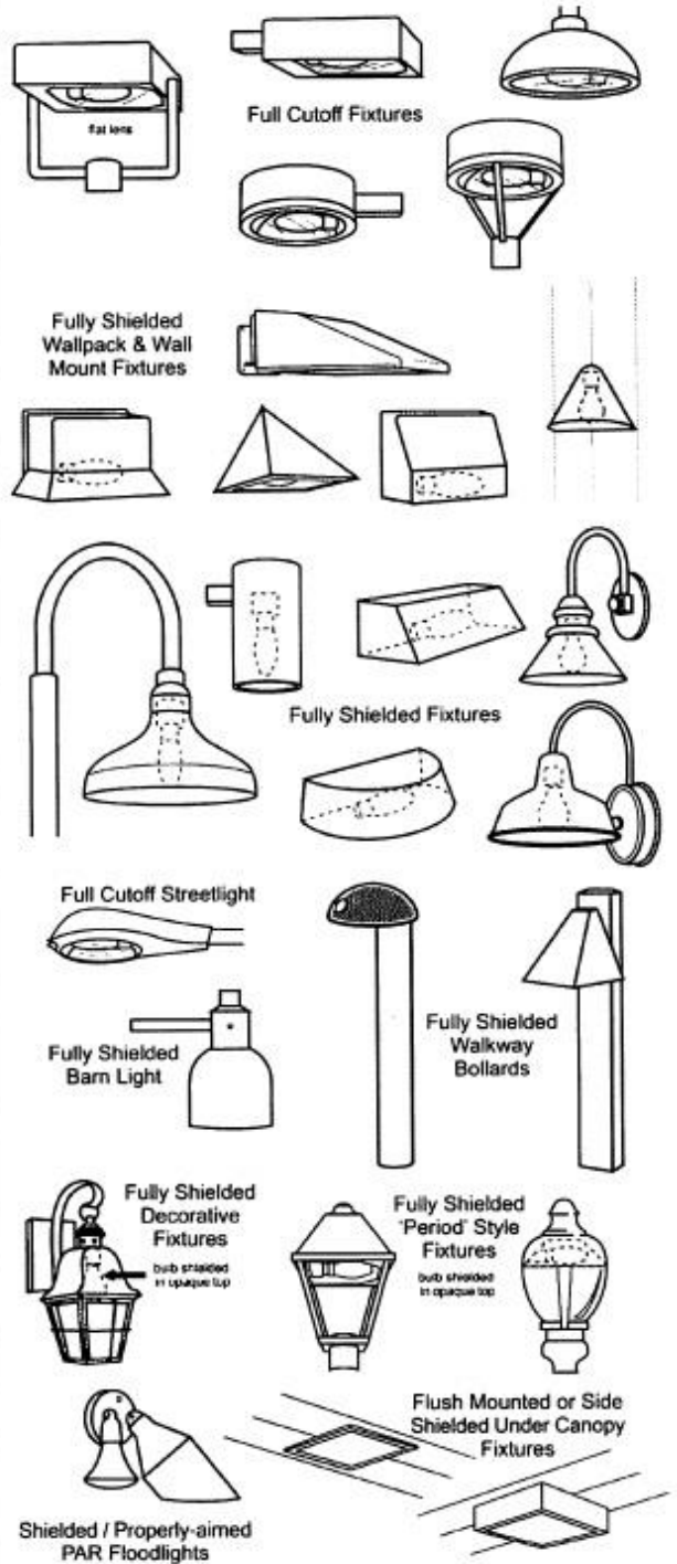
Figure B: Examples of Unacceptable/Noncompliant Fixtures and Acceptable/Compliant Fixtures.
